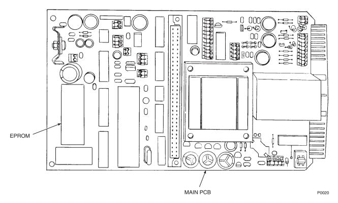
Figure 2-10. Main PCB (Model 218A) EPROM Replacement
